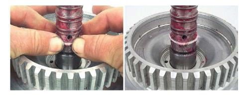
• This is the part where you can carve up the ring if you're not very careful. Slide the ring sizer tool down the turbine shaft until it contacts the top seal ring. Very gently push down on the sizer while moving the top of the sizer tool from side to side, and around in circles. This helps gently feed the ring into the groove.
