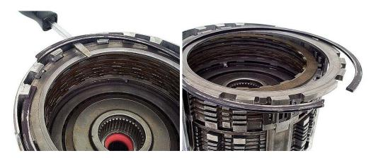
**Step 5:** Remove the 3-4 clutch snap ring and selective pressure plate.
