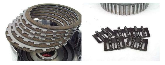
**Step 7:** Remove the 3-4 clutch apply plate. There may be either a single or double apply plate assembly, depending on model.
