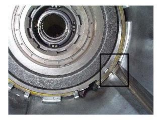
**Step 34:** Slide the output shaft back into the rear of the case. Using a soft mallet, tap on the rear end of the output shaft to knock the low roller clutch out of the case lugs. Once the roller clutch assembly is clear of the lugs, remove the output shaft from the case. Reach into the case and remove the low roller clutch from the case.
