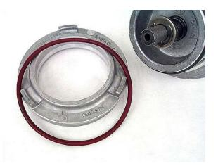
**Step 16:** Remove the seal rings from the  $2^{nd}$  gear piston. Remove the e-clip from the servo pin, then slide the washer and spring off of the pin.
