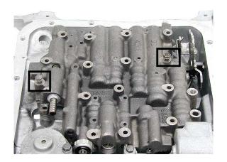
**Step 56:** Place a new o-ring on the end of the TCC solenoid. Install the solenoid, making sure that the wires aim toward the valve body. Tighten the bolts good and snug.
