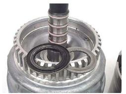
Step 22: Remove the turbine shaft o-ring.
