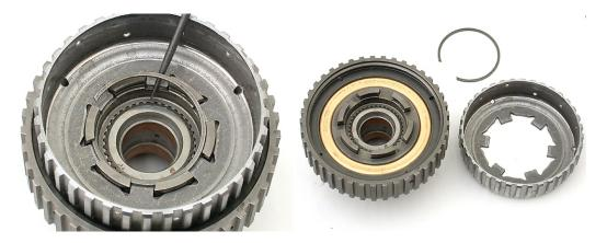
**Step 10:** Lift the sprag outer race from the assembly. Separate the sprag element and end plates from the inner race. Inspect both sprag races for wear or scoring. Inspect clutch hub teeth for wear.
