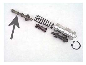
**Step 39:** Before assembling the boost valve and sleeve, drill the hole in the boost sleeve as shown to 0.042" (#60 drill) to improve line pressure response time. Make absolutely sure that there are no burrs left inside the sleeve from the drilling operation.
