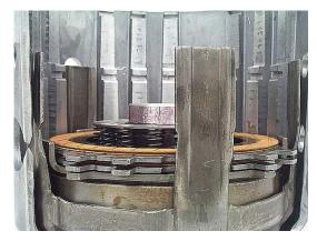
**NOTE:** There are several types of steel plates used in the input drum that are very similar, but will not interchange. The correct plates must be installed in the correct locations. Use this illustration to determine correct plate location. The plates are shown in their proper respective position within the input drum.
