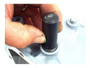
• Coat the manual shaft with assembly lube, then slide it partway into the case bore. Position the manual lever as shown, and start the manual shaft through it.
