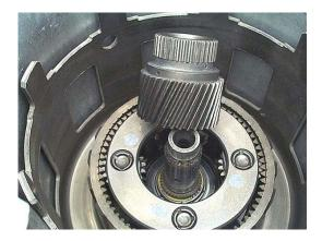
**Step 29:** Hold the output shaft up into the case with one hand while using a pair of small thin snap ring pliers to remove the output shaft snap ring from above the front planet. It may seem a bit like a juggling act, but you don't want the output shaft to hit your toe when you remove the snap ring. It hurts. Once the snap ring is off, slide the output shaft out of the case.
