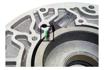
**Step 25:** Pressing the slide toward the side seals to compress the rubber support strip, install the pump slide swivel pin spring and swivel pin.
