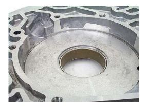
**CAUTION:** Make certain that you wipe off **any** excess locking compound from the bushing after pressing it into place. If any of this compound gets into the pump rotor area, a destroyed pump is practically assured.
