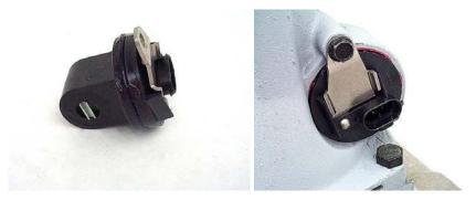
If the unit came to you with a range sensor and/or an external shift lever bolted to the manual shaft, install them now. Transmission assembly is now complete.
