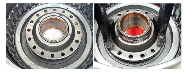
Step 9: Place the cushion plate onto the piston, dished side down.
