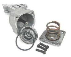
**Step 5:** Inspect the press fit of the piston pin to the bottom of the accumulator housing bore. There must be no gaps or looseness.
