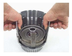
**Step 8:** You will need to help the inside piston seal over the last bump in the drum with a feeler blade or other suitable tool. Once the piston has cleared the last bump and is in the proper position, you will see about 3/16" of drum above the seal below the first step. When you press down on the piston, it will spring back a little bit. Coat the seal bore in the top of the forward piston with assembly lube.
