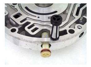
**Step 36:** Install the line pressure blow-off ball and spring into the proper hole in the stator support. Push the spring in with a suitable tapered tool, and install the retaining pin to hold the spring in place. Make sure that the pin head goes below flush with the pump surface.
