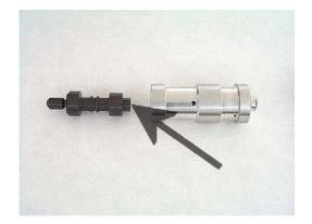
**Step 41:** Slide the pressure regulator valve and pressure regulator valve springs into the pressure regulator bore.
