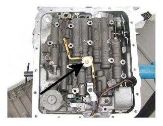
Step 59: Install the auxiliary valve body tube and the two tube hold-down brackets.
