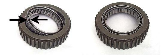
Step 20: Place an end bearing on the inner sprag race as shown.
