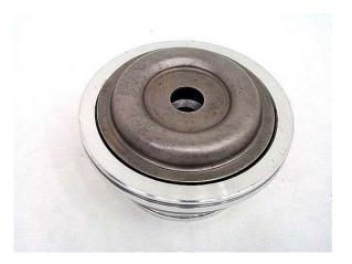
**Step 21:** Press down on the retainer plate, then install the snap ring to hold the plate into the piston.
