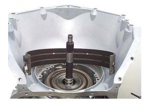
• Align the case anchor end of the band with the anchor hole in the case, then slide that end of the band between the case and the reverse drum until the anchor end of the band is over the anchor hole in the case. You can help position the band by pushing on it through the case passage next to the manual lever.
