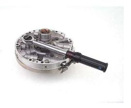
**IMPORTANT:** After the pump body and stator support are bolted together, make sure that the rotor can be turned by hand using the pump shaft, a converter hub, a pick or other suitable tool. Be very careful not to nick the front seal or bushing. If the rotor won't turn, disassemble and re-check your slide and rotor clearances.
