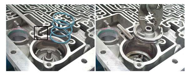
Step 18: Use a magnet to remove the 2-4 band anchor plug from the case.
