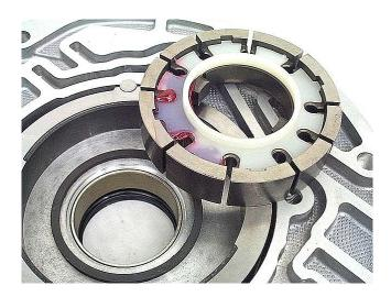
Step 28: Place the rotor into the pump pocket (guide ring down, if equipped).
