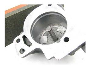
**Step 16:** Place a new seal on the piston. Coat the housing and pin with assembly lube. Install the piston and spring into the housing.
