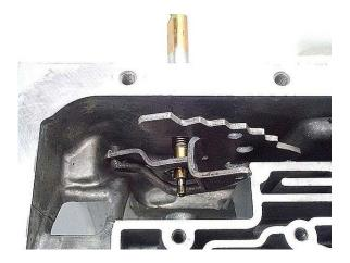
• Place the manual lever retaining nut over the end of the shaft, then slide the shaft the rest of the way into the case. Tighten the manual lever nut firmly.
