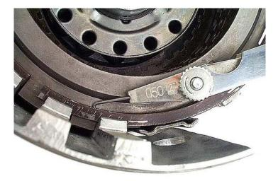
**Step 18:** Once proper clearance has been checked and corrected if necessary, remove the forward pressure plate and snap ring. Install the lube seal into the drum against the inner end of the turbine shaft. Place the thrust bearing as shown on top of the lube seal, using assembly lube to hold it in place.
