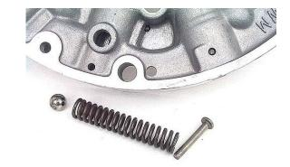
**Step 17:** Gently flat sand the passage walls of the pump, as well as the stator support passages if equipped, only enough to get rid of high spots around bolt holes and edges. Inspect all pump parts for wear or damage, replacing any bad parts you may find. Thoroughly clean all pump parts.
