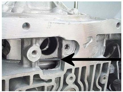
**Step 31:** Put new o-rings the pump bolts, coat the top of the pump bolt holes with assembly lube, then install the bolts into the case.
