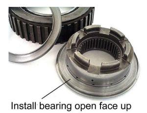
**Step 21:** Install the inner race into the sprag as shown by rotating the inner race counterclockwise.
