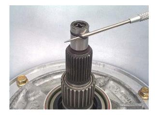
**Step 23:** Remove the front seal. It's much easier now, with the weight of the unit holding the pump still, than it will be later.
