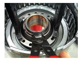
**Step 4:** Remove the return spring assembly from the drum. Remove the piston, and take the lip seals off of the piston.
