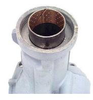
Step 29: Coat the outside diameter of a new rear seal and drive it into the housing.
