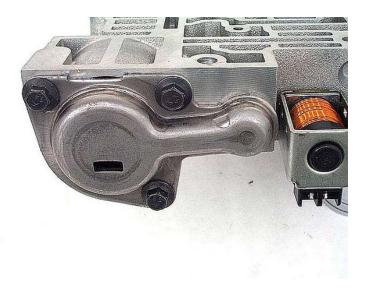
**Step 13:** Remove the 1-2 accumulator piston and spring from the accumulator housing, taking notice of which order they came out of the housing in. Remove the seal from the piston. Clean all accumulator parts.
