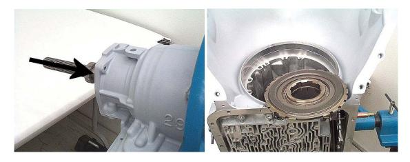
**Step 35:** Remove the rear planet from the case. Some of the low-reverse clutch plates may come out with it.
