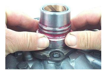
• After you've squished the ring into the groove as best as you can, center the ring in the groove and slide the ring sizer tool over the ring groove area.
