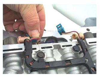
Step 10: Remove the manual lever detent spring.
