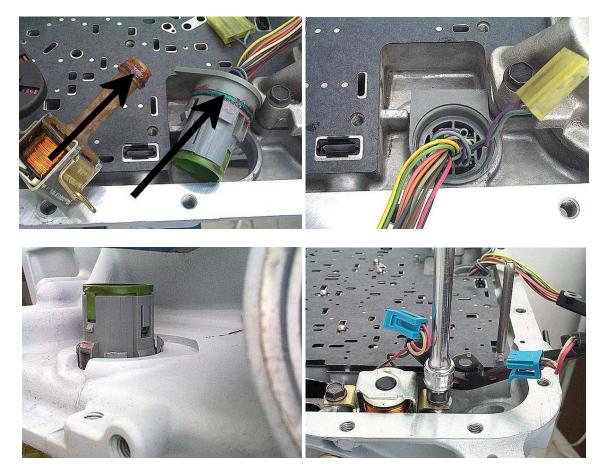
**Step 48:** Pull the wiring harness away from the valve body gasket, then carefully lower the valve body onto the case. You must guide the free end of the manual valve link into position in the end of the manual valve along the way.
