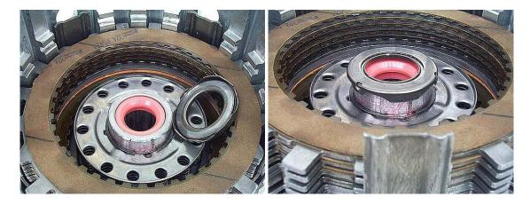
**Step 19:** Install the input sprag into the drum (which is shown being serviced in the Gear Train section), feeding it through both sets of clutches. You will know when the sprag is all the way down against the thrust bearing when you can push down on the sprag and still turn it easily in both directions. Once the sprag is in place, re-install the forward clutch pressure plate and snap ring.
