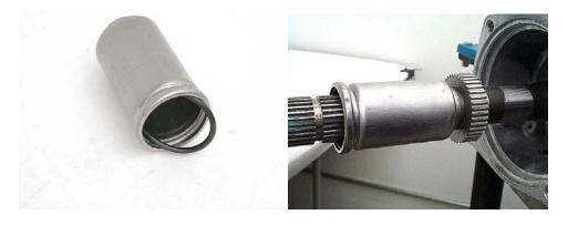
**Step 68:** Install a new lathe-cut seal on the extension housing if one hasn't already been installed. Make sure that the extension housing's speed sensor or speedometer cable adapter hole is aimed toward the same side of the case that the manual shaft is on, then tap the extension housing into place on the back of the case. Torque the four housing bolts to 26 ft-lbs.
