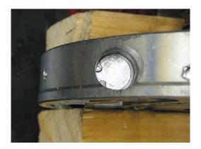
**Step 49, 4L60E only:** Use the appropriate size bushing driver to install a new filter neck seal into the filter bore of the stator support.
