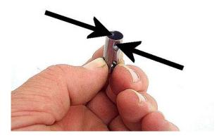
**Step 9:** blow any metal chips out of the capsule hole. Place a new checkball capsule into the hole, *open end up*. Use a 3/8" driver or a long 3/8" bolt with the threads cut off to drive the capsule into position.
