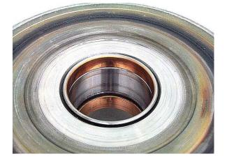
Place the appropriate thrust washer on the stator support, and set the reverse input drum on the support. Check the top drum bushing for clearance. There must be no more than 0.003" clearance between the bushing and the journal. Check the drum for any side-to-side or rocking motion. If there is any motion, replace the drum bushings. Be sure to chamfer the edge of the larger bushing after installation to help the drum go over the seal rings during unit assembly.
