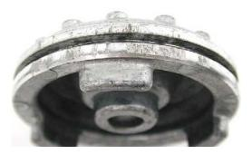
**Step 15:** Make sure that there is no wear on the pin. If wear is found, the housing must be replaced. Resurface the piston bore and pin with ScotchBrite <sup>TM</sup>, then flat sand the mounting surface of the housing. Thoroughly clean the housing and piston.
