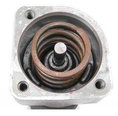
**IMPORTANT:** The cover must have an oblong hole over the pin that the pin must *not* be able to fit through. If you have an earlier cover with a round hole, it *must* be replaced.
