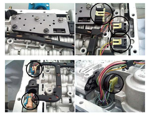
**Step 50:** Place the proper bolts through the harness hold-down eyes. Remove the alignment pins, then install the proper bolts into the remaining holes as shown, remembering to install the dipstick stop clip on the front corner of the valve body.
