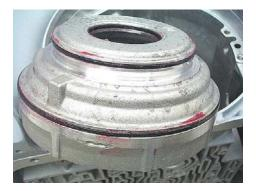
**Step 2:** Coat the seals and case bores with assembly lube. Line up the piston lug with the proper slot in the case. It might be easier to line up the lug with the slot if you make a mark on top of the piston where the lug is.
