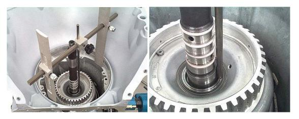
• Place a new pump gasket on the pump, and place the inverted 'H' gauge on the gasket. Use a feeler gauge to measure the clearance between the gauge pin and the thrust journal on the end of the stator support. This clearance, minus two or three thousandths, is your endplay distance.
