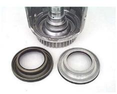
**Step 14:** Remove the forward piston housing inner o-ring from the input drum. All input drum parts are now ready for cleaning and inspection.
