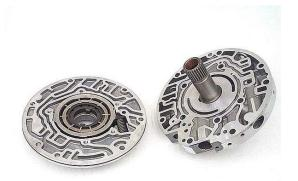
Step 6: Remove the top pump vane ring (which may be sticking to the stator support.
