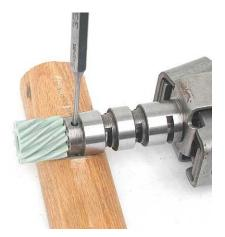
**Step 20:** Pull the gear out of the shaft. Use a small screwdriver to also pry the valve out of the governor shaft. Thoroughly clean the governor parts.
