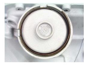
**Step 37:** Insert the 3-4 accumulator piston pin into the 3-4 accumulator bore in the case. Place a new seal on the 3-4 accumulator piston. Smear some assembly lube inside the 3-4 accumulator bore. Install the 3-4 accumulator piston into the case, open side up. Install the 3-4 accumulator spring into the piston. Place checkball #91 into position in the case pocket next to the 3-4 accumulator as shown.
