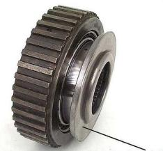
Rotate inner race counter-clockwise to install
