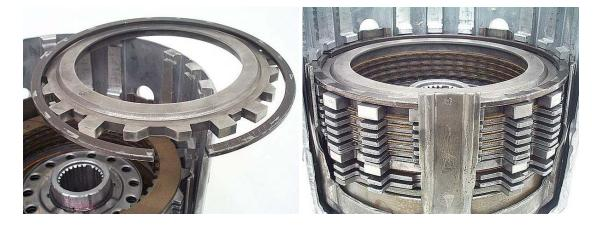
**Step 17:** Measure the forward clutch clearance between the pressure plate and the snap ring. The clearance should be 0.030"-0.063" (0.75mm-1.60mm). Adjust the clearance by changing the forward clutch pressure plate, which comes in the following sizes:
