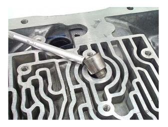
**Step 19:** If you haven't already done so, remove the manual valve link from the manual valve lever.
