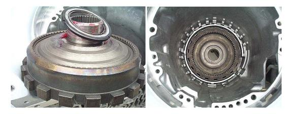
**Step 8:** Place the rear planetary assembly rear thrust bearing into position on the back of the rear planetary assembly as shown, using assembly lube to hold the bearing in place. Lower the planetary assembly into the rear ring gear, engaging the ring gear teeth.
