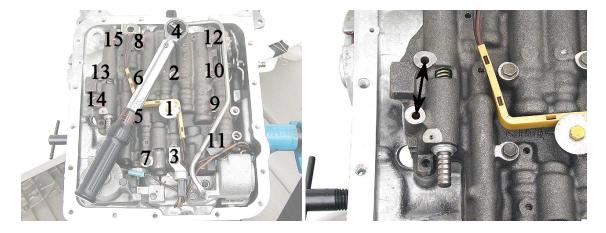
**Step 61:** Connect any switches that still need to be hooked up, then install the manual lever detent spring and tighten the bolt good and snug.
