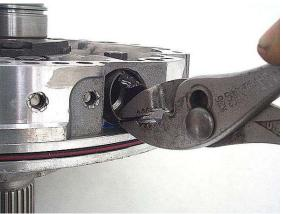
**Step 2:** Remove the pressure regulator boost valve retaining snap ring (4L60E shown). The boost valve and pressure regulator valve assembly should pop out of the pump. Later, when the pump halves are separated, you can gently push or pry any parts out of the bore that don't want to come out peaceful-like.
