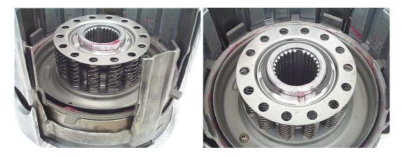
**Step 11:** Using an appropriate compressing tool, compress the overrun return spring assembly far enough to install the snap ring. Make sure that the ring goes inside of all four snap ring retaining tabs on the spring assembly.
