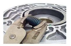
• Holding the springs over the pocket, tap the springs with a small hammer. This should knock the springs from the grips to the pocket, leaving your forehead or glasses intact.
