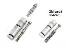
• Replacing bore plugs with both a stock TCC shift valve *and* installing a TCC shift TV valve update kit.
