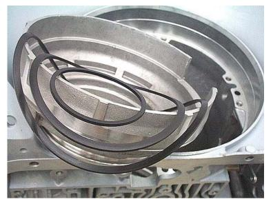
**Step 40:** Evaluate the condition of the major components inside the unit. If no major components need to be replaced, and **Step #21** showed that you needed to adjust endplay, now is the time to get the correct endplay shim for the input drum. If endplay was too great, you need a thicker shim. If endplay was too little, you need a thinner shim.
