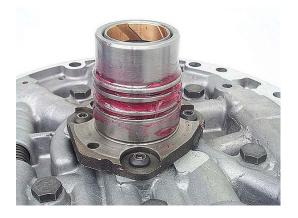
• Place the ring expander tool over the stator support tower, lining up the bottom of the tool with the top of the lower seal ring groove. Quickly slide a new ring down the tool until it pops into the lower groove.
