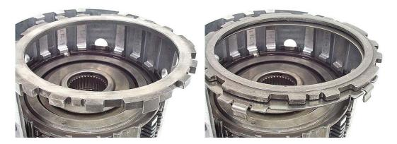
**Step 8:** Remove the forward clutch snap ring and pressure plate. This is one of the toughest snap rings you'll ever encounter, so expect some fighting with a screwdriver to get it out. Try not to beat up the drum too badly in the process.
