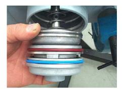
• The recommended service tool for this procedure bolts to the pan rail and compresses the servo piston as you tighten the tool bolt.
