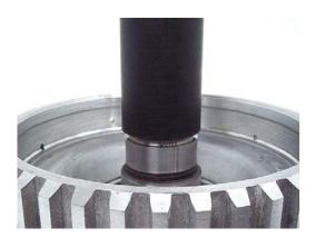
• Quickly slide a new seal ring down the tool until it pops into the ring groove.
