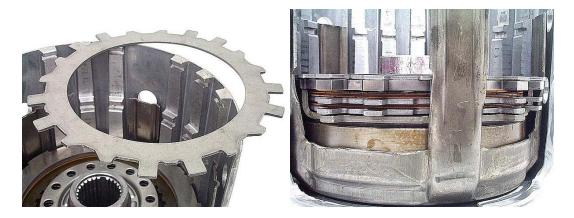
**Step 15:** Install the forward clutch plates, starting with a steel plate against the waved plate.
