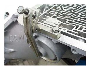
• A large pair of channel-lock pliers placed over the pan rail and against the servo cover will provide constant inward pressure on the cover while you gently tap on the other side of the cover. Be very careful not to damage the pan rail with the pliers.
