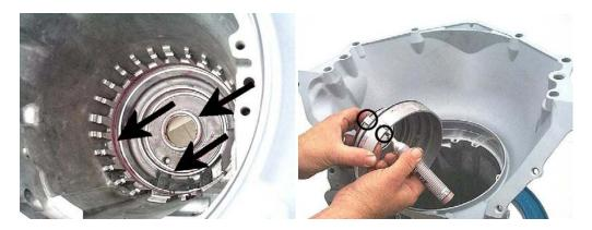
**Step 3:** Using a hammer handle, gently tap the piston into position in the case bore. Be extremely careful, because these seals rip very easily during installation, and ripped low-reverse seals are one of the most common after rebuild complaints for this unit. You will know when the piston is all the way down when you can see the outer seal bore above the edge of the piston near the park pawl.
