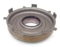
**Step 6:** Place the 3-4 clutch apply ring on the bench. Set the 3-4 clutch return spring assembly inside the apply ring. Place the forward piston and housing assembly on top of the 3-4 clutch return spring assembly, lining up the wide lugs on top of the forward piston with the fingers of the 3-4 clutch apply ring.
