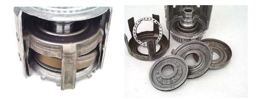
**NOTE:** Don't worry about the condition of the forward piston, or bother removing the lip seals from it. One of the most common 4L60E failures is a cracked aluminum forward piston, so during the Input Drum Assembly section you will be instructed to throw this piston in the trash, replacing it with a steel piston with molded seals.
