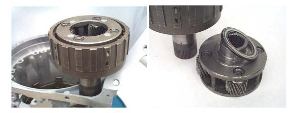
**Step 31:** Lift the sun gear shell out of the case and remove the metal thrust washer from the inside of the sun gear shell. Locate and retrieve the plastic thrust washer that was *under* the shell. It may have stuck to the backside of the shell or may be sitting on the low roller clutch inner race.
