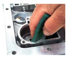
**Step 12:** Flat sand the valve body surface of the case, and remove any pump gasket material from the pump surface of the case.
