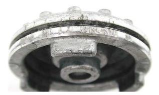
**Step 7:** Resurface the piston bore and pin with ScotchBrite <sup>TM</sup>. Make sure that there is no wear on the pin.
