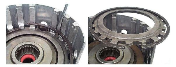
**Step 9:** Remove the forward sprag assembly. Remove the thrust bearing and lube seal from the input drum.
