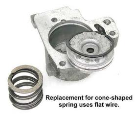
**NOTE:** If the 1-2 accumulator uses a cone-shaped spring, it must be replaced with the new style spring available from your parts supplier.
