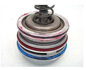
**IMPORTANT-** If the servo teflon ring sticks too far out of its groove, it's sure to get cut to pieces during servo installation. This is one of the most common rebuild errors made on this unit.
