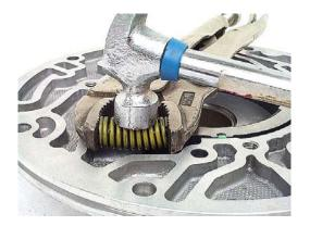
• After the spring pops into the pocket, be sure to press the spring with your thumbs all the way below flush with the top of the spring pocket.
