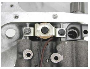
**NOTE:** Some model valve bodies have a TCC switch that may interfere with tightening the solenoid bolts. Lift the valve body a little bit to gain access to the bolts with a wrench.
