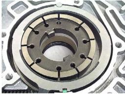
Step 29: If you are using used pump vanes, find the side of each vane that has two 'rub marks' from riding against the vane rings, and aim that side of each vane toward the center of the rotor. Install half of the pump vanes in a semi-circle, making sure that the vanes don't go on top of the bottom vane ring.
