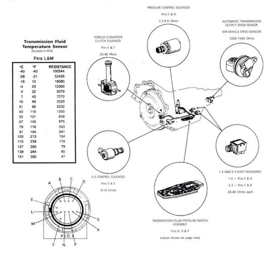
In order to properly test the Transmission Fluid Pressure Switch Assembly, the engine must be running and under full computer control (all wiring connected). Since the computer is sending 12 volts to each of these switches, the resistance of the switches can not be checked with an ohmmeter. Use a voltmeter and check for the proper voltage on the appropriate harness wires in each of the shift lever positions (the wires will need to be pierced).
