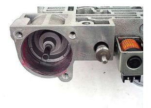
Step 11: Install the accumulator spring and the low overrun valve spring.
