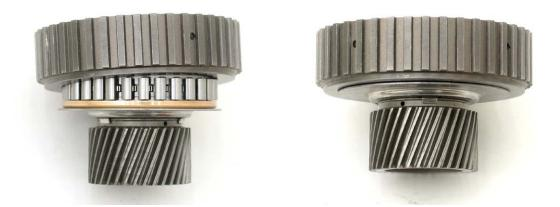
Step 14: Place the second sprag end bearing onto the sprag element.
