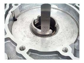
**NOTE:** New bushings may have a high durability coating on the inside of the bushing. These coatings usually have a dark gray or light green color. These coated bushings have been working quite well, so it is a good idea to use this type bushing to avoid friction damage and a spun bushing.
