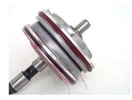
**Step 25:** Coat the 4<sup>th</sup> piston seal ring groove with assembly lube, then install the seal ring into the groove. Place the 4<sup>th</sup> piston over the flat end of the servo pin as shown, with the larger-bump side of the 4<sup>th</sup> piston facing away from the 2<sup>nd</sup> piston.
