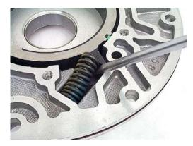
**Step 10:** Remove the pump slide from the pump pocket. Inspect the bottom of the pump pocket and the side of the pump pocket where the slide side seals rub. If there is any noticeable wear or scoring, the pump body must be replaced. Remove the slide side seals and slide top or bottom seal ring and rubber support ring. If the seal ring sticks in place, use an air nozzle to shoot air under/around it to unseat it.
