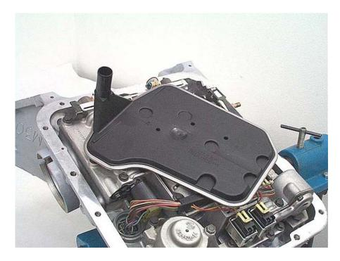
Step 9: Disconnect the electrical wiring from the solenoids and the pressure switch assembly.
