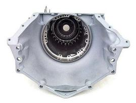
**Step 2:** Inspect the internal case lugs for wear or damage where the low roller clutch assembly contacts the lugs. If there is more than 1/16" lug wear, the case should be replaced. Although there are repair devices made to correct this wear problem on the THM350, don't use them on the 4L60E. The 4L60E has a much lower first gear, and under high load could break the repair devices and the case.
