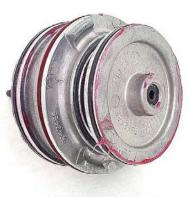
**Step 26:** Place a new rubber 0-ring (the larger of the two servo o-rings) into the servo cover groove. Place the servo cover over the  $4^{th}$  piston, being careful to guide the seal ring into the cover without cutting the ring. Slide the servo return spring over the pointed end of the servo pin.
