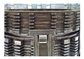
**IMPORTANT:** The 3-4 clutch steel plates have teeth of different widths around the plate, which must be installed into the drum in the proper manner in order to allow room for the 3-4 clutch boost springs. All wide steel plate teeth must go into narrow drum slots only, and pairs of narrow teeth must go into common wide drum slots only.
