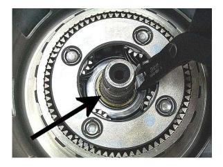
**Step 23:** Place the front sun gear into the front planetary carrier, shoulder side up, engaging the teeth of the front planetary gears.
