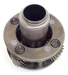
**NOTE:** Thrust bearings should not be run through a cleaning machine unless they are trapped within an assembly. Cleaning machine deposits can remain in the bearings, causing rapid wear and failure.
