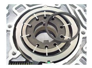
**Step 7:** Lift out the pump rotor. There may be a plastic pump vane guide ring either in the pump pocket or stuck to the pump rotor. Remove this guide ring.
