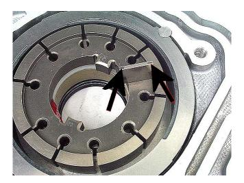
Step 30: Using a pick in a vane slot, push the bottom vane ring against the installed vanes. This should provide enough clearance to install the rest of the vanes.
