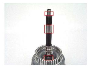
**Step 3:** Remove the four teflon seal rings from the turbine shaft. Since there must be absolutely no damage to the sides of the ring grooves, the best way to remove the rings is to stab them through the middle with a pick. This breaks the ring without touching the side of the ring groove.
