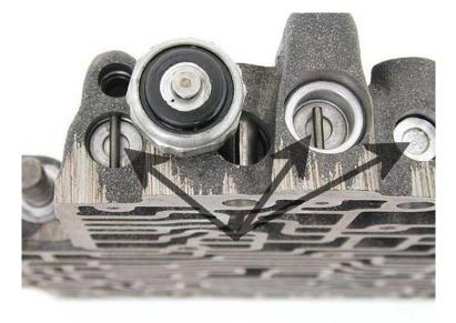
**Step 2:** The throttle valve is prone to sticking, causing late or no upshifts. Therefore, we recommend that you install an anti-stick spring over the inner end of the throttle valve, available through most transmission parts suppliers. Make sure that the small end goes over the valve, with the large end pointing toward the bottom of the valve bore.
