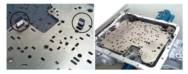
**Step 42:** Place the valve body gasket (identified by a 'V' cut into the gasket) on top of the separator plate.
