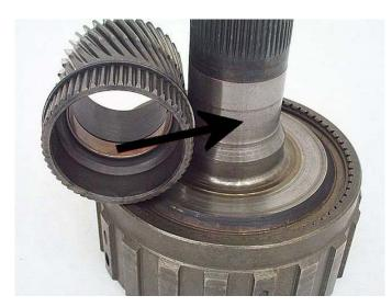
**Step 4:** Inspect all thrust surfaces for wear or scoring. Thrust surface discoloring is usually normal, and is not cause for replacement of the part. However, just like the bushing journals, if you can feel the wear there's too much there. These surfaces can also be reconditioned using ScotchBrite<sup>TM</sup> or #400 grit emery cloth.
