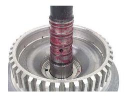
• Place the seal ring installer over the turbine shaft, adjusting the tool height adjustment bolt so that the bottom of the tool lines up with the top of the lowest empty seal ring groove.
