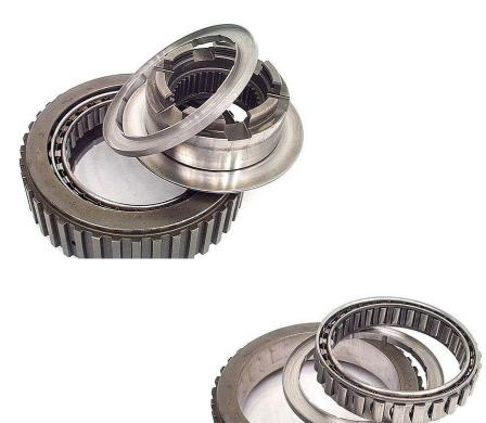
**Step 18:** Use #240 grit emery cloth to break through the glaze on both inner and outer sprag races. Finish both surfaces with #320 grit emery cloth. Thoroughly clean all sprag components.
