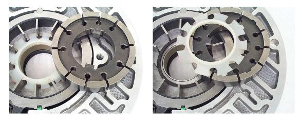
Step 8: Remove the pump rotor vanes and bottom vane guide ring.
