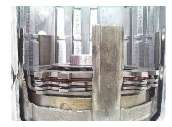
Step 14: Install the forward clutch waved plate.
