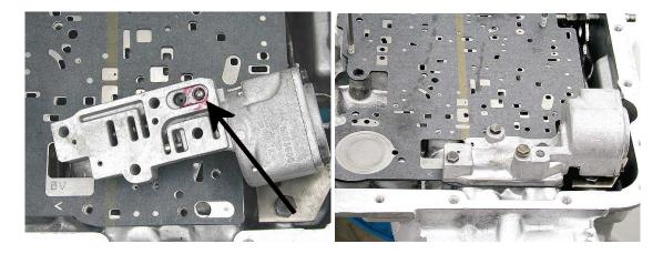
**Step 44:** Place the 1-2 accumulator housing on the separator plate, install the proper bolts, then tighten bolts to 8 ft-lbs.
