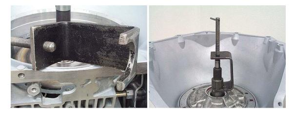
If you are going to pry the pump out rather than using a puller, be careful. Gently pry in several places, including the area between the reverse input drum and the pump.
