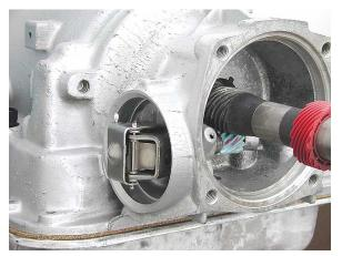
**Step 65:** Place a new lathe-cut seal on the governor cover. Install the cover onto the case, making sure that any removal dents on the cover flange are aiming toward the rear of the case. Gently tap the cover into position with a hammer until it fully seals against the case. Use a large punch or a socket extension to bang any dents on the flange flat.
