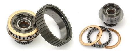
**Step 11:** Use #240 grit emery cloth to break through the glaze on both inner and outer sprag races. Finish both surfaces with #320 grit emery cloth. Thoroughly clean all sprag components.
