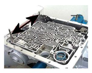
Step 40: Place the case gasket (identified by a 'C' cut into the gasket) on the case.
