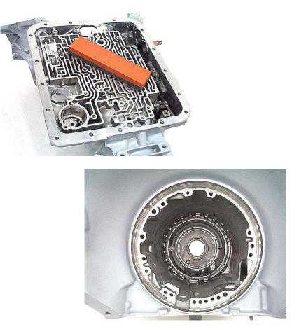
**Step 13:** Thoroughly clean the case. Blow any standing water or cleaning solution out of the case passages rather than let it drip dry. This keeps any cleaning machine deposits from contaminating the new ATF or causing valves to stick after the unit goes back into the vehicle.
