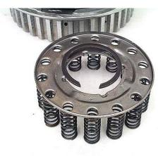
**Step 12:** Grab the drum by the turbine shaft, flip it over and slam it against the bench again. Isn't transmission rebuilding fun? All piston assemblies except for the 3-4 piston should fall out of the drum. Separate the forward and overrun piston assemblies, and remove the lip seals from the overrun piston.
