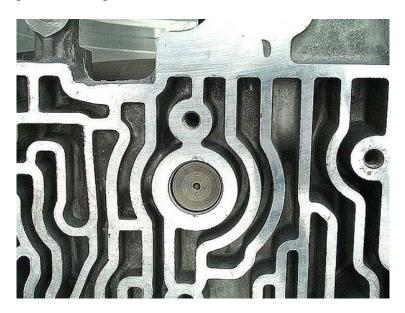
**Step 29:** Place the pump gasket into position on the case. Thread a pair of pump alignment pins into two pump bolt holes across from each other. You can make alignment pins out of two long 8mm bolts that fit the pump bolt holes in the case that you have cut the heads off of, rounded the cut end, then cut a screwdriver slot into.
