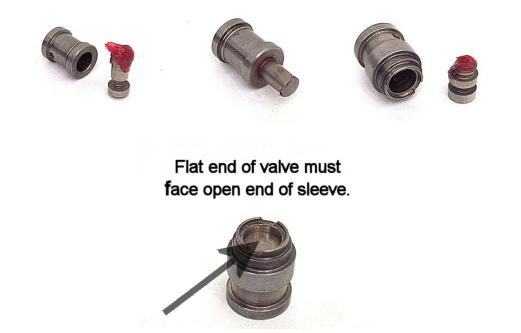
**Step 45:** Slide the pressure regulator valve and spring into the stator support, making sure that it slides freely the full length of its travel.
