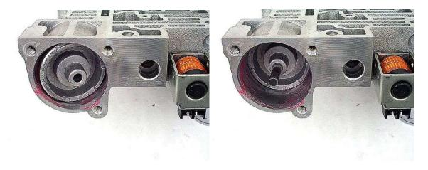
Step 10: Install the low overrun valve into its bore.
