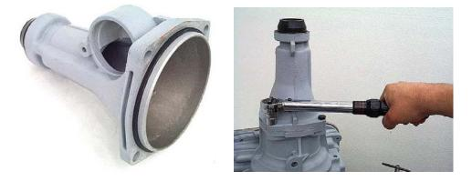
**Step 69:** Put a new o-ring on the output speed sensor, then slide the sensor into the extension housing and tighten the sensor bolt to 8 ft-lbs.
