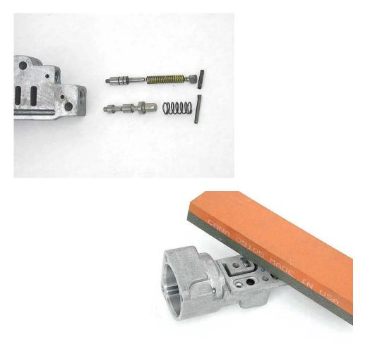
**Step 9:** Thoroughly clean all parts. Be sure that the forward clutch apply orifice is not restricted.
