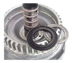
**Step 2:** Inspect the three turbine shaft bushing journals for wear or damage. If problems are found, replace the drum.
