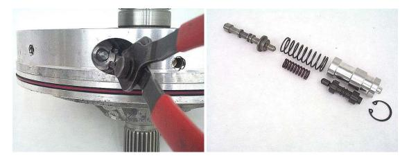
**Step 3:** Remove the TCC apply valve retaining snap ring from the valve bore. The retaining plate, valve and springs should fall out of the bore.
