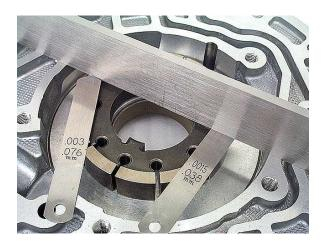
**Step 20:** Remove the rotor. Place the slide swivel pin into its pocket. Lower the slide into the pump body where it normally rides against the swivel pin. Lay a straight edge across the slide. Measure the clearance between the straight edge and the slide at several points around the slide. The clearance must be between 0.002"-0.003".
