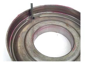
**Step 5:** Install a new forward steel piston into the piston housing. Although you may need a feeler blade to help push the seal into the housing, it can usually be installed by hand without tools. Try pushing the lip in with your thumbnail, if you have one.
