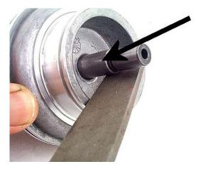
**Step 18:** Use a small screwdriver to pry one end of the snap ring out of the  $2^{nd}$  gear servo piston. Press down on the spring retainer plate and remove the snap ring. Remove the cushion spring retainer and spring.
