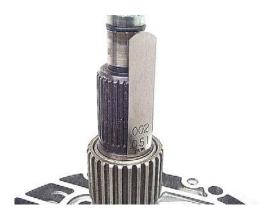
**Step 33:** Always replace the rear stator bushing. This bushing is responsible for maintaining centerline throughout the transmission more than any other bushing, and is subject to rather high loads.
