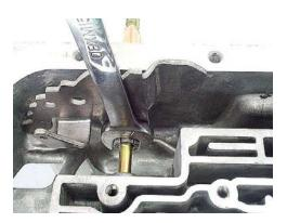
• Pry the manual lever toward the center of the case to provide access to the manual shaft clip, then pry the manual shaft clip off of the manual shaft.
