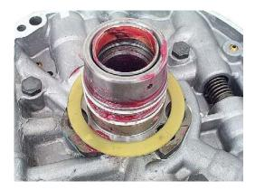
**Step 55:** Install the pump o-ring into the pump body groove without twisting it, making sure that the line on the OD of the ring is visible all the way around the pump.
