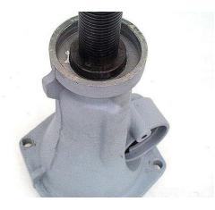
**Step 28:** Install a new bushing into the extension housing, being careful not to drive the bushing in at an angle. An arbor press is best to assure good alignment. You can use an old driveshaft yoke to check for proper bushing clearance.
