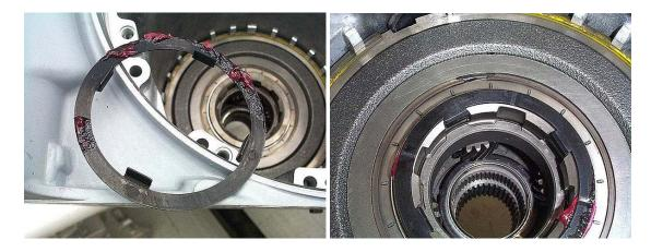
Step 15: Install the rear sun gear into the rear planetary carrier.
