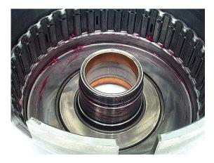
**Step 7:** Install new lip seals on the reverse input piston, then install the piston into the drum. Use a feeler blade or other suitable tool to guide the seal lips into the bores. Be very careful not to cut the seals.
