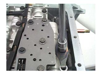
**Step 11:** Remove the pressure switch assembly. Inspect the underside of the switch assembly for ripped seals or particle contamination within the switch. Replace the assembly if any of these problems are found.
