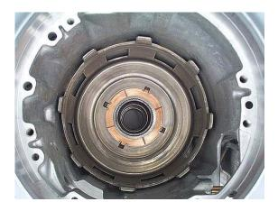
**Step 18:** Place the front planetary carrier rear thrust bearing in position on the back of the planetary carrier, using assembly lube to hold the bearing in place. Install the planetary carrier into the front ring gear and hub assembly.
