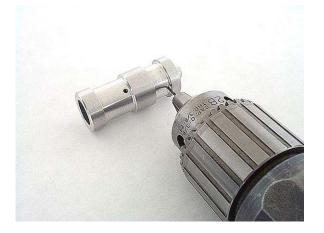
**Step 40:** Smear some assembly lube on the inner end of the boost valve, then slide the pressure regulator boost valve into the sleeve.
