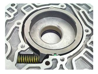
• Smooth out any burrs or dents that the grips may have left on the pump walls.
