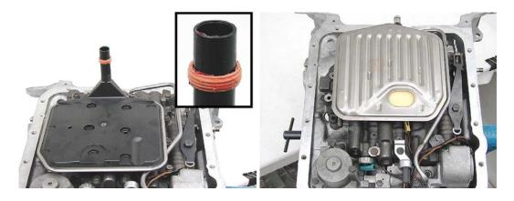
**Step 63:** Place the magnet in the correct position in the pan. Install a new pan gasket on the case pan rail, then lower the pan onto the pan rail.
