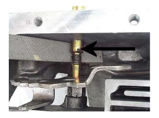
• Remove the manual shaft from the case and smooth the area of the shaft where the seal rides with some ScotchBrite<sup>TM</sup> or #400 grit emery cloth.
