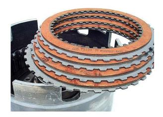
**Step 11:** Install the selective pressure plate and snap ring into the drum.
