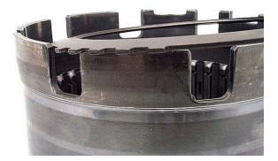
**Step 10:** Load the clutch plates into the drum, starting with a steel plate, ending with a friction plate.
