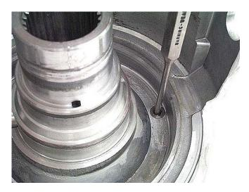
**Step 2:** Install the forward piston housing inner o-ring into the input drum groove as shown. This is usually a green o-ring in most kits. Coat the ring with assembly lube. Coat the drum center tower and 3-4 piston bore with assembly lube.
