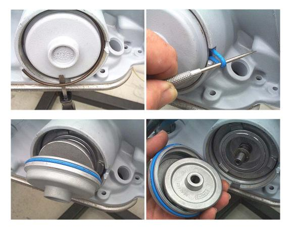
**Step 6:** Remove the rest of the servo components from the servo bore. If the servo assembly appears stuck, carefully pull on the servo pin snap ring with a pair of pliers.
