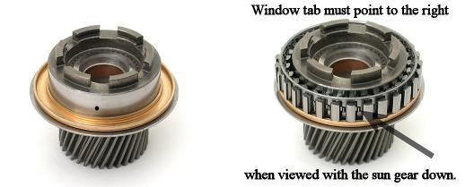
**Step 13:** Start the sprag outer race over the sprag element at an angle, rotating the outer race counter-clockwise when viewed with outer race on top. You'll need to push the last few teeth into the outer race with your finger as you rotate the outer race.
