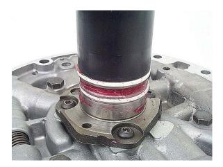
**Step 54:** Place the reverse input drum thrust washer into position on the stator support using assembly lube to hold it in place.
