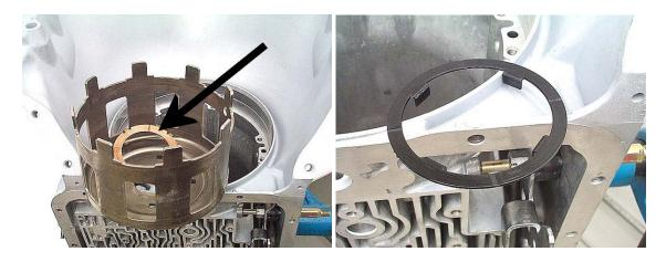
Step 32: Remove the rear sun gear from the rear planet.
