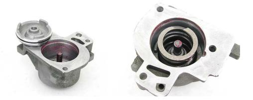
**NOTE:** The spring and piston position may be reversed on your model. Install the parts in the same direction they came out.
