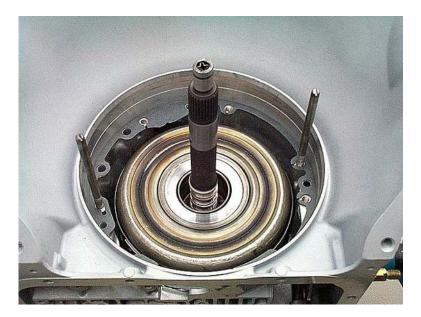
**NOTE:** It is a good idea to run a thin bead of high quality silicone sealer around the outside of the pump o-ring just before you install the pump into the case.
