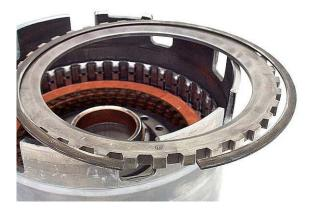
**Step 12:** Measure the clutch clearance between the pressure plate and the snap ring. This clearance must be between 0.040" and 0.076" (1.02mm-1.94mm). If your clearance is not within these specifications, adjust the clearance by installing the correct pressure plate. The available pressure plate thicknesses are:
