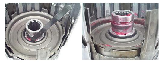
**Step 9:** Install the overrun piston into the forward piston, using a feeler blade to guide the inner piston seal over the snap ring groove in the drum tower. When fully installed, the piston should appear in the position shown.
